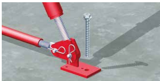
Assembling of supporting props
